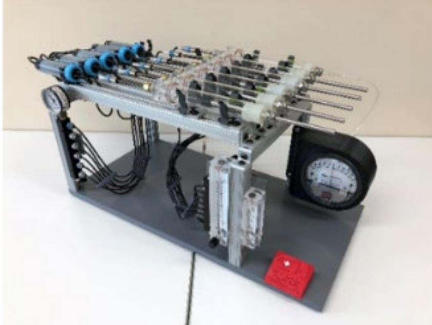
Final six tube rack system
